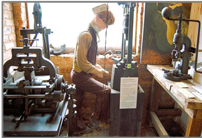
Stamping out the needle eyes using a foot operated press.
