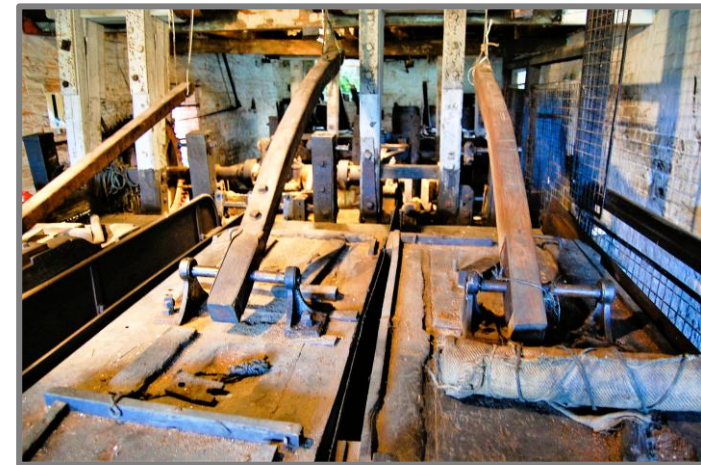
The water powered scouring beds used to clean and polish the needles.
