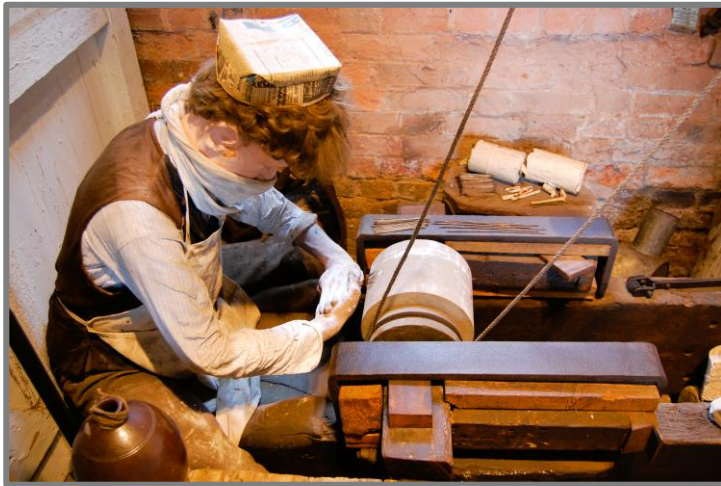
Needle Pointing using a water powered high speed rotary grindstone
